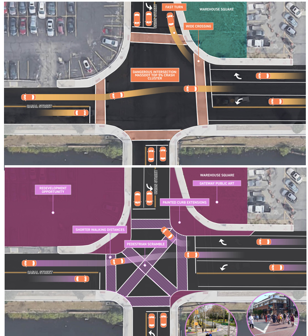
Diagram of conditions (top) and proposed safety improvements (bottom) at Union and Canal Streets
